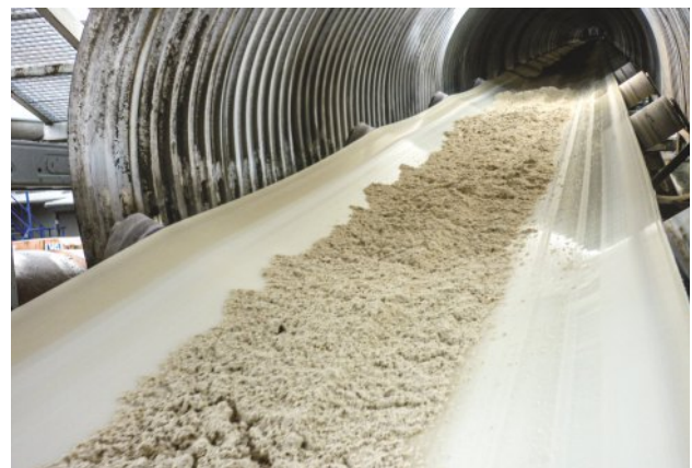
After: The PVG 70 system prevents material from migrating into the lower belt
