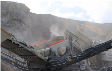
Multi-use for primary scalping and screening.
