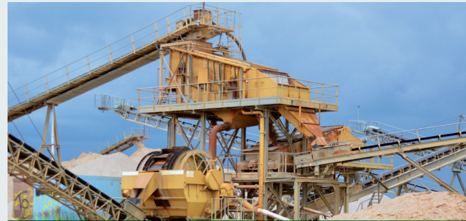
STICHWEH preparation plant with DOUBLE-DECK SCREENING MACHINE VS 24/60 Twin-shaft log washer DSW 150/2100/6000 Bucket wheel ES 3509 BB
