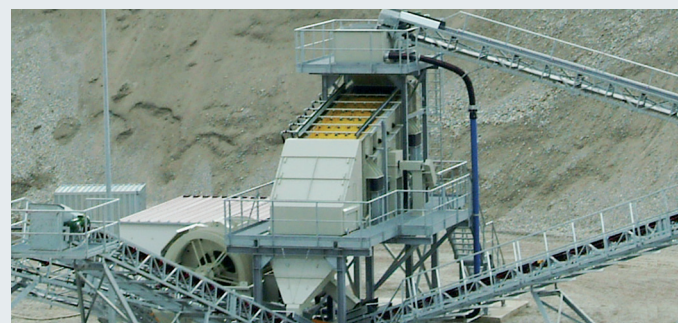
STICHWEH preparation plant with SINGLE-DECK SCREENING MACHINE VS 15/40 THREE-DECK SCREENING MACHINE VS 18/60 Bucket wheel ES 3009 BB
