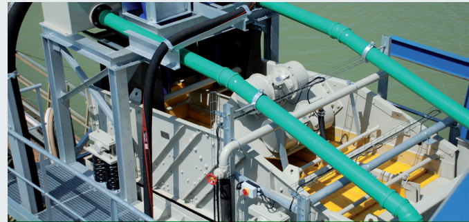
STICHWEH DEWATERING SCREENING MACHINE EB 18/35 with 2 screening decks and cyclone
