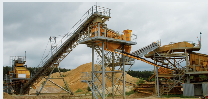
STICHWEH preparation plant with SINGLE-DECK SCREENING MACHINE VS 15/40 DOUBLE-DECK SCREENING MACHINE VS 24/60 THREE-DECK SCREENING MACHINE VS 15/50 Twin-shaft log washer DSW 120/2100/6000 Dewatering screen Eb 09-25-1
