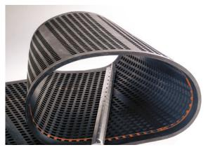
For both cross- and length-tensioned screens, our Sandvik WX6000 tensioned rubber panels are designed with precision-punched holes for fine- to medium-coarse screening in your dry applications. Its flexible rubber reduces the risk of pegging and blinding, and it is hardwearing with strong, heat-treated cord reinforcement near the bottom of the panel to extend its wear life.
