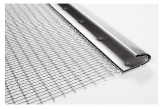
This is a tensioned screening media used primarily for fine to medium screening in dry applications. Generally with separations between 1-90 mm and max. feed lump size at 200 mm.
