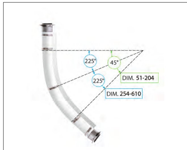
INSIDE - Recommended number of clamps, support beams placed on the inside of the hose bend.
