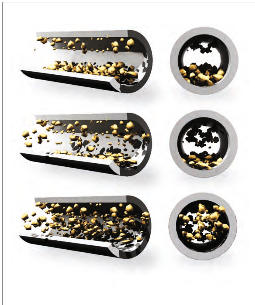
Different flow conditions. The third (lowest) variant in the figure represents the preferred flow condition.
